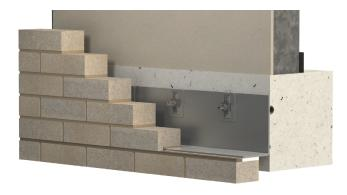
For scenarios where the cavity size is less than 50mm, a T2 system can be utilised. This basic system is used where there is no availability to fit a bracket into the cavity size. Due to the larger bending moment upon the angle at larger cavities, T2 systems become uneconomical and should be replaced with a T1 bracket and angle system.
