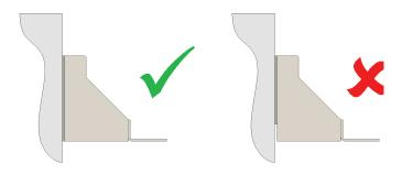
The maximum allowable thickness of the shims should not exceed the outside diameter of the fixing. As ACS Masonry Support systems typically utilise 12mm diameter fixings, this tends to be the maximum allowance. If more than 1No. shim is required, it is important that the total number of shims is kept to a minimum to avoid creating slip planes that may allow settlement or creep under load.
